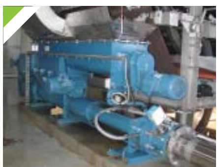
GBB pump for recovery of sticky sludge with belt filter and lubrication
