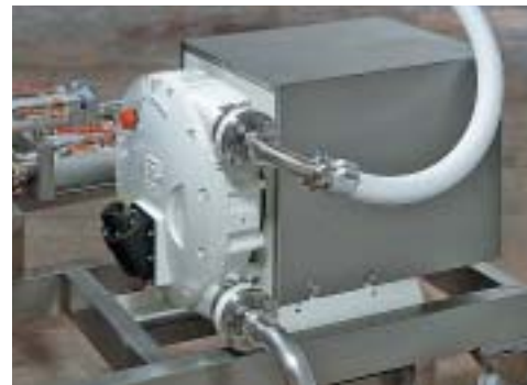
DL Pump in the ready-made meals industry: racking from a mobile tank into hopper of a dosing system supplying the container packing line
