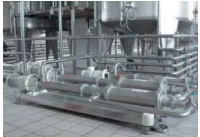
Moineau Series H Pumps with fresh dairy products: Plain bulk yogurt transferred to heat-exchanger and then to packing line
